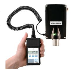
work and settings can be made from ground level. The display of the RC2 remote control shows the same information as would be shown by the EC28 versions with display. This makes inspection, maintenance and calibration much easier.
