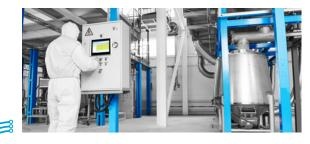
Controllers are the local control center and data hub of integrated gas detection systems. They turn the data from transmitters into actions. In turn, controllers allow the collected information to be further stored or evaluated by a higher order processing or data center. GfG offers a wide range of controllers for various applications.
