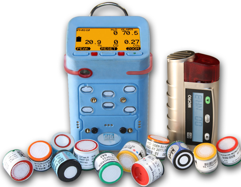
Figure 2: Compact electrochemical (EC) sensors are available for an increasing number of specific toxic gases. Ammonia sensors show very little response to interfering gases, are capable of low ppm range resolution, require very little power, and are comparatively inexpensive.
