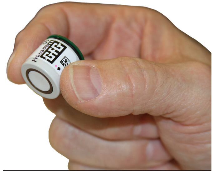
Figure 1: Compact electrochemical ammonia sensors exhibit excellent linearity, are capable of low ppm range resolution, and are comparatively inexpensive.
