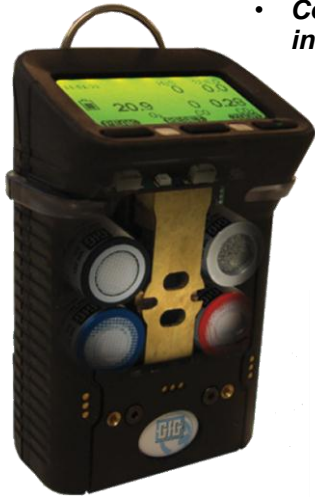
GfG IR sensor (Note longer pathlength)
